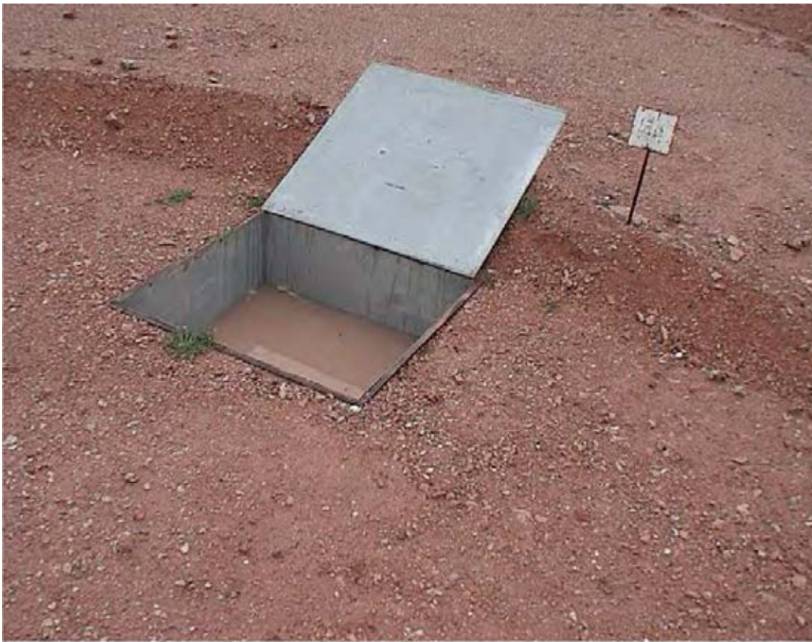
Soil erosion and runoff traps
